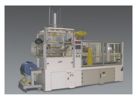
**AC** is a universal continuous cycle thermoforming machine for the positive and negative molding of material in coils that can be adapted to the thermoforming of thermoplastic materials in sheets.
